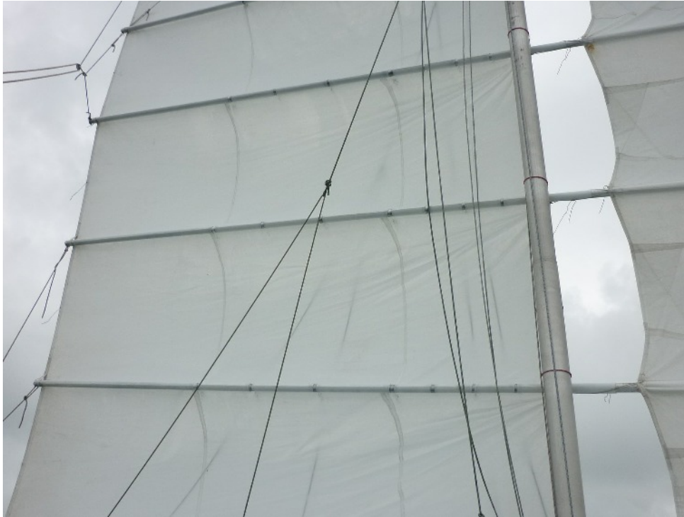
The 'Broadening' of the seams in the main panels can be seen as they approach the batten at the top of each panel. Note the lack of rope work compared to many other junk rigs, with only the spare halyard and the slack yard hauling parrel adding to the halyard and lazyjacks.
