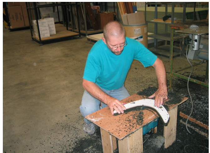
Using a template to router the rough-cut noses to shape and round off their edges:
