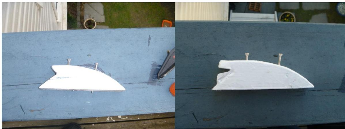
**The core of Frøken Sørensen's tiller brake, before and after modification to a narrower notch.**
