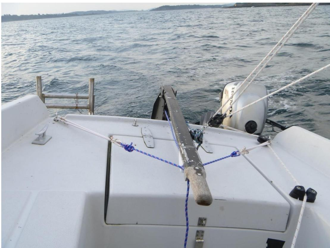
The 6.5m Jollenkreuzer, *Frøken Sørensen* steering herself well - as long as the apparent wind is from ahead, and the wind strength doesn't vary too much...
