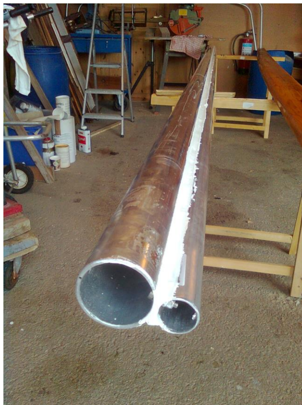
20160528 Ingeborg's yard bolted and epoxied together, with the epoxy string covered with 2-pot paint. Dimensions, main tube: 65 x 3.5mm, upper tube: 35 x 2mm.
