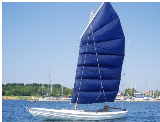
..18ft dinghy Broremann with 10sqm sail. Note the mast lift and simple lazy jacks...
