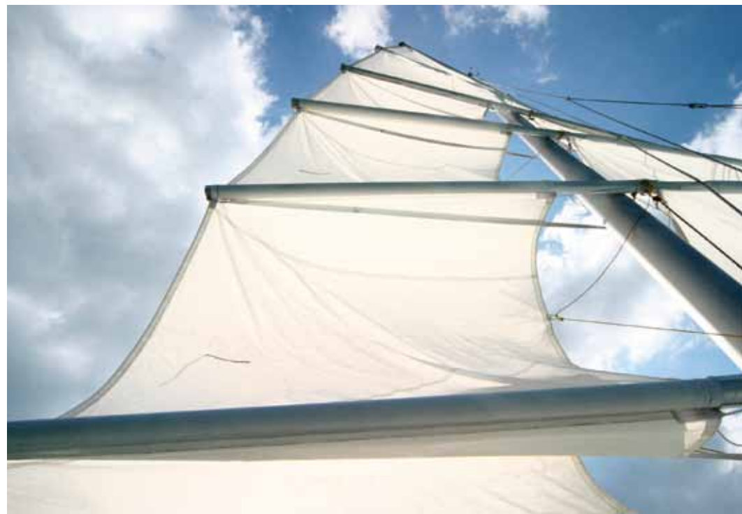
Splitting the rig: the jiblets at work forward of the mast in the lower five panels of the seven-panel sail
