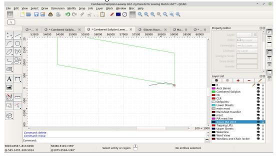
Use the rotate command to align the bottom of the airfoil with the panel edge (use the arrow selection to and snap the rotation to the line that is the bottom of the panel).
