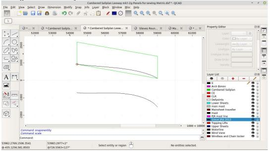
This time we also use the Mirror command to copy the airfoil to the top of the panel (mirror axis is middle of luff and leach), and then the Move command to snap it into its proper place in the corner.
