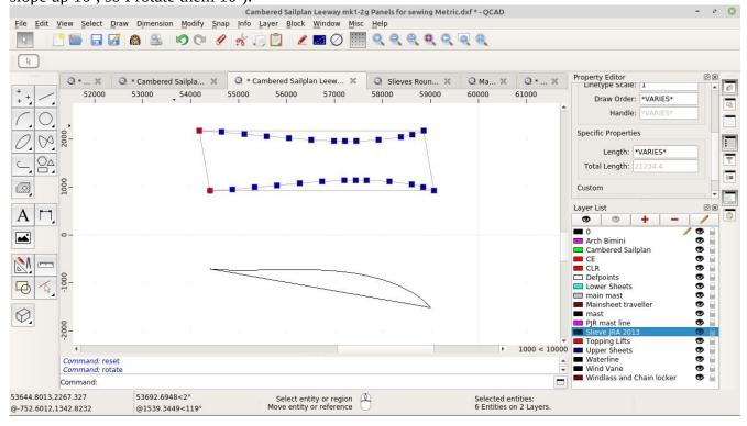
The length of the top of my airfoil was 4793 and my panel length along the batten was 4674 so 4792.5/4673.6 = 1.025. So, we now scale the panel in the x-axis only by 1.025. To finish rotate the panel back to its original angle (-10°), and you have now completed a panel and shelf foot for your 8% camber panel.
