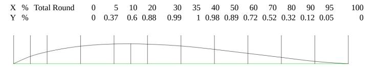
I have one base airfoil I'm using and I drew it to 6% camber (it's maximum thickness is 6% of its length from luff to leach). So, the first thing I needed to do for the lower panel was increase this to 8% camber. To do this use the Scale tool and scale only the y-axis by 8/6 (1.333).
