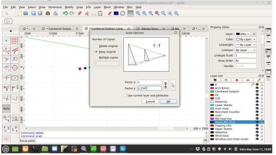
Use the move command to bring the forward end of the airfoil to the forward end of the panel.
