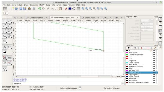
I used the airfoil Slieve provided in the JRA magazine (Feb 2013 JRA Issue 61). There, he provided it to calculate how much rounding you add to a barrel rounded panel, but if you use the maximum camber you want for your airfoil it plots an airfoil that seems as good as any without a wind tunnel to test with. It also has shape that thinks about how the actual sail will set when made with cloth that will stretch a
