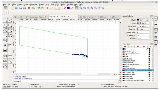
Now make the airfoil bottom the same length as the panel edge. Use Scale, use the front edge of the panel as your anchor point, and use the pointer (rather than specifying an value) to drag your airfoil to the opposite corner of the panel.
